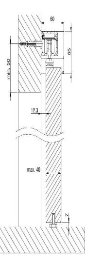
Rail Type Profile Wall Mounted Height Adjustable 60 kg Max Door Weight Min Door Width 850 mm Suitable for Wooden Doors Min Wooden Door Thickness 34mm Max Wooden Door Thickness 40mm SSO Finish Rail Dimensions (WxH) 60 x 65 mm 1 Leaf Option Soft Close Standard Length 2000mm Optional Length (special order) 2500mm **DIN EN 1527** 100,000 cycles Wall Distance (door-wall) Wood 5.5mm Optional Skirting/Architrave Spacer Kit 12.5mm
