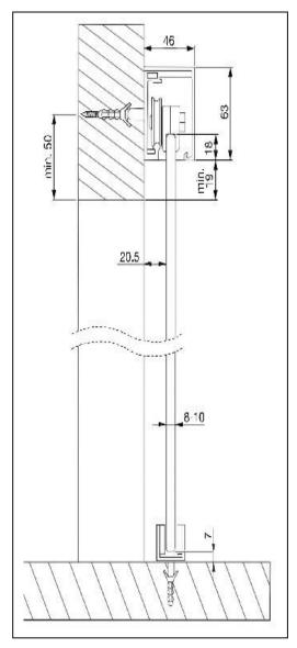
Rail Type **Profile** Wall Mounted Height Adjustable Max Door Weight 60 kg Min Door Width 850 mm Suitable for 8mm Glass Suitable for 10mm Glass Suitable for Wooden Doors no Finish SSO Rail Dimensions (WxH) 46 x 63 mm 1 Leaf Option 2 Leaf Option Soft Close
